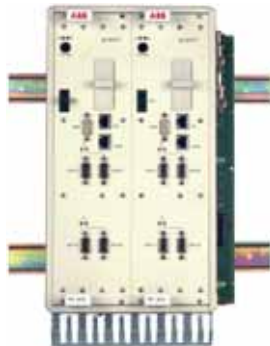
Figure 10: The AC 870P CPU Housing
