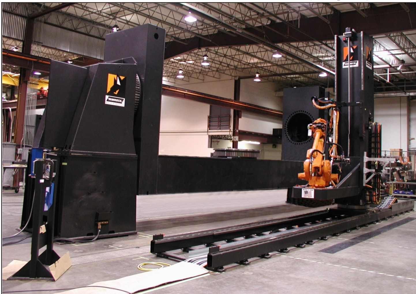
The IRB 4400L robot welds engine end frames on the drop center H positioner of the robot cell while traveling along the track on a robot rotating tower.
