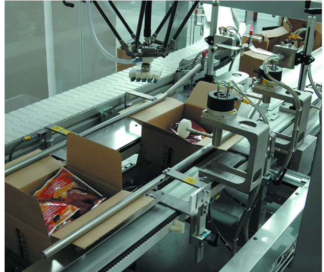
The Skinetta end-of-line packaging machine packages up to 88 bags per minute. The RobTeq Speed-Picker packages bags weighing up to 1,000 g. The suction technology of the ABB FlexPicker was optimised in order to achieve this.
