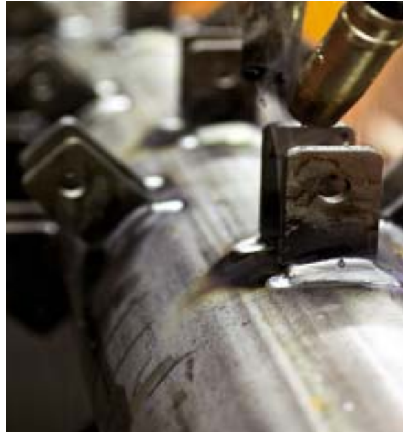
With the ABB robot, Kverneland now have one process, compared with four in terms of welding the rotor.
