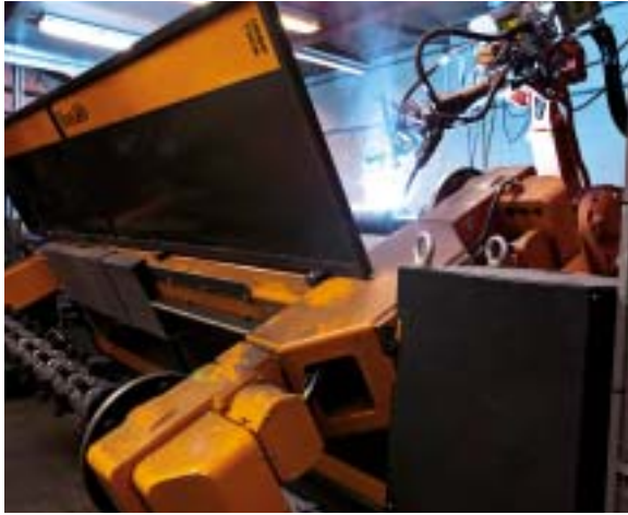
With the ABB robot, Kverneland now have one process, compared with four in terms of welding the rotor.
