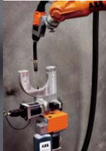
A TSC, Torch Service Center, with BullsEye precision is a valuable feature in Krog Iversen's new robot system for automatic welding.
