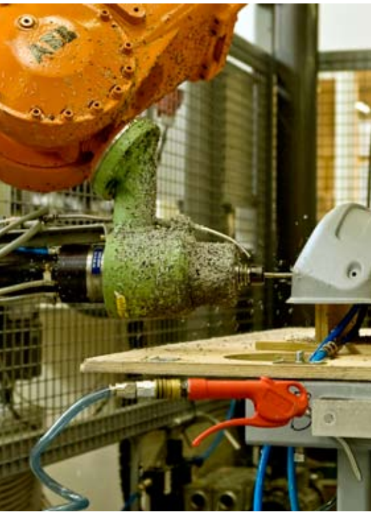
With robots, 150 parts per hour can be sawed versus 15 when done manually.
