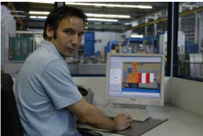
Offline programming on the factory floor: Detlef Wittke creates robot programs in RobotStudio ArcWeld PowerPac.
