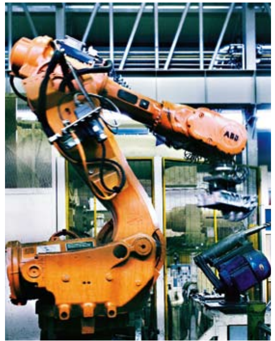
An IRB 6650 can handle 30 components per hour, compared with 10 when handled manually.
