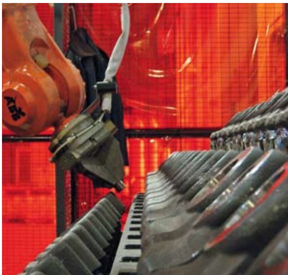
The operation to place and weld the teeth takes 10 hours, manually the process would take up to 100 hours.
