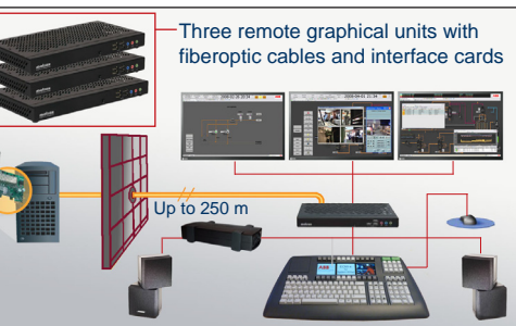
3 All client computers remotely connected via fiber optic cables
