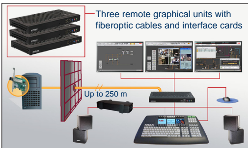
3 All client computers remotely connected via fiber optic cables
