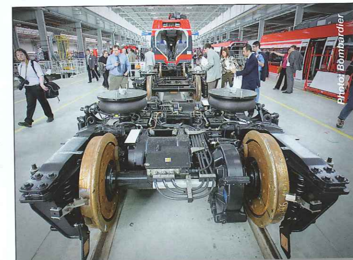
The Talent 2 runs on bogies from the Flex-Compact family, like those on which the AGC and Spacium are mounted. The primary suspension system comprises rubber bushes and steel springs with a vertical shock absorber on its outer side.
