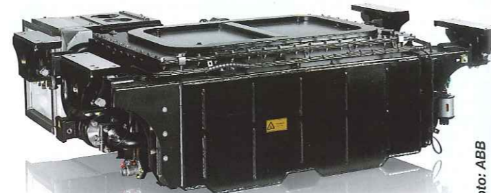
A two-traction winding Class A traction transformer for Talent 2 EMUs. It is designed to operate off 15 kV 16.7 Hz, giving an output of 856 kVA, its short circuit voltage is 22 %, and at 85 °C its losses are 62 kW. The cooling medium is mineral oil, the maximum oil temperature is +105 °C, the minimum service temperature is -25 °C. The transformer measures 2,654 x 2,341.5 x 806.5 mm, and it weighs 3,800 kg. It incorporates an oil pump, three flange valves, three oil drain screws, an Elastimold high voltage bushing, four low voltage Pfisterer and one DIN bushings, and one overpressure valve. Protection against radio interference is incorporated.
