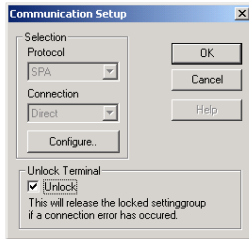
Figure 33: Communication setup dialog for release of the locked setting group.
